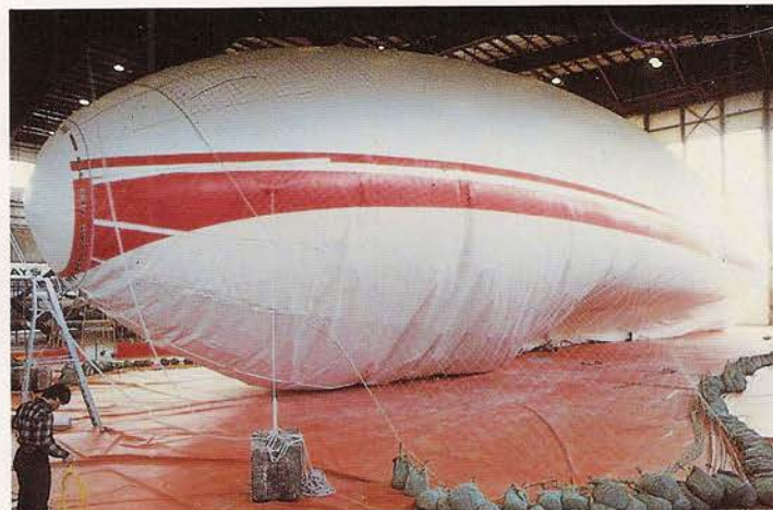
Skyships building. Top, a gondola moulding is prepared by Slingsby Aviation Ltd., of Yorkshire. Centre, inflation of a Skyship envelope and below, looking much like an enormous model kit, one of the more recent Skyships (G-SKSL) nears completion in Japan.
