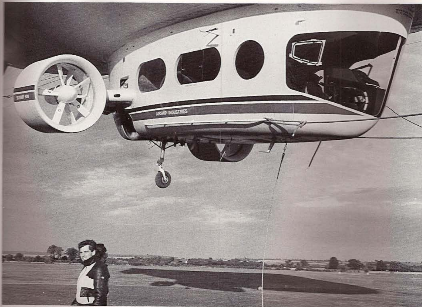
Right, pilot David Griffiths awaits final clearance for take-off from Radlett aerodrome during London Skycruise, July 1987. Below, 500-02 shows its single-wheel undercarriage strut to advantage as the ship 'kites' at the mast on a blustery day.
